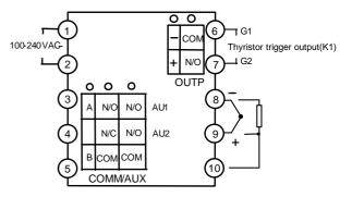
control. If I2 module is installed with bAud = 1, it simulates MIO slot to read on-off input (terminals 3 and 5) to switch between SP1/SP2 or switch the program status RUN / Stop (AI-526P).
