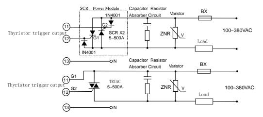
**Note 1:** According to the voltage and current of load, choose a suitable varistor to protect the thyristor. A resistor-capacitor circuit (RC circuit) is needed for inductance load or phase-shift trigger output.
