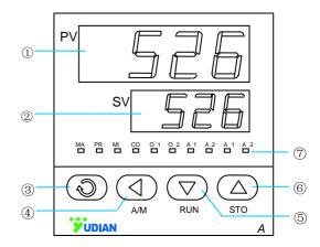
**Basic display status :** When power is on, the upper display shows the process value (PV) and the lower display shows the set point (SV). At certain circumstances, the lower display blinks SV and the following status message. The symbol message.
