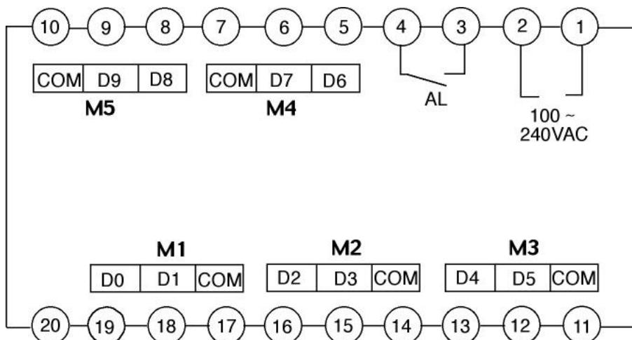
D0-D7 for external alarm switches inputs. D8 is for silencer switch input, and D9 for test switch input. AL is for relay output. ALL the COMs are the common terminals and internally connected.
