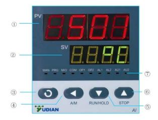
① Indicator lamps: OP1 and OP2 indicate the status of current retransmission. AL1, AL2, AU1and AU2 indicate the I/O actions of the corresponding modules.
