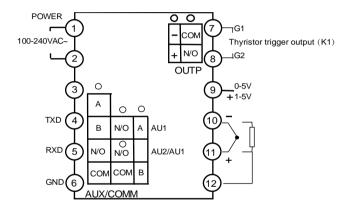
Wiring diagram of dimension D7 (22.5 x 100mm)
