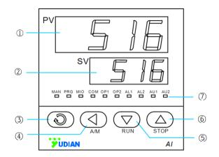
When power is on, the upper display shows the process value (PV) and the lower display shows the set point (SV). At certain circumstances, the lower display blinks SV and the following status message. The symbol message:
