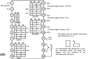
Wiring diagram of rear terminals of short depth
