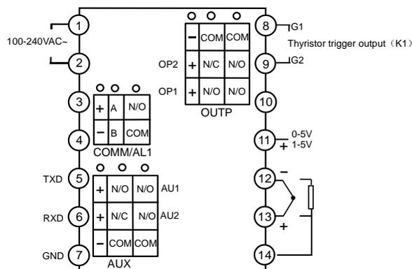
Note 1: Linear voltage signal of range below 500mV should be inputted from terminals 13 and 12, and signal of 0~5V and 1~5V should be inputted from terminals 11 and 12.
