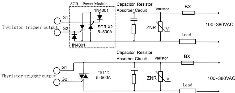
Note 1: According to the voltage and current of load, choose suitable varistor to prevent the thyristor. Capacitor resistor absorber is needed for inductance load or phase-shift trigger output.
