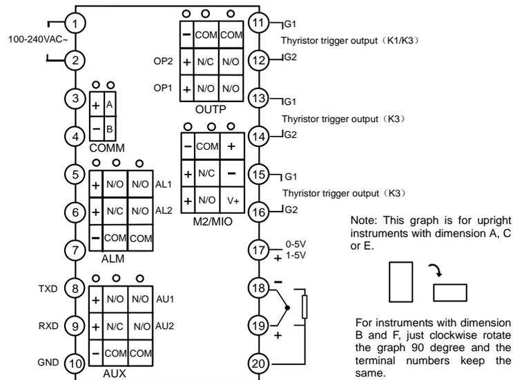
Note 1: For linear voltage input, if the range is below 500mV, connect to terminals 19 and 18. 0~5V or 1~5V signal can be inputted from terminals 17 and 18.
