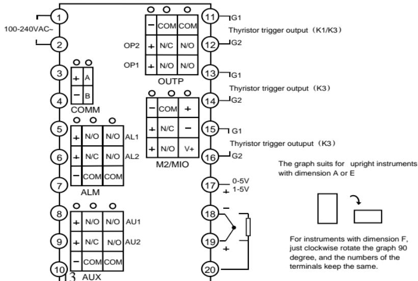
should be directly connect to the terminals. When the internal auto compensation mode is used, connecting the common wire between the compensation wire and the terminals will cause measurement error.
