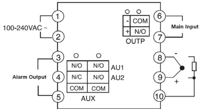
**Wiring graph for D dimension (72mm X 72mm) instruments**
