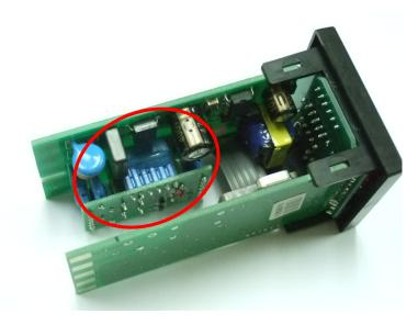
5. Modules unplugged. Usually the module number is printed on the left bottom corner. Some will be printed on label instead.
