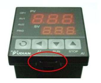
2. The panel with PCBs can be slide out easily. During pushing back, a "click" sound is heard when the knot is locked.
