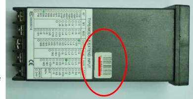
If the serial number is lost or worn out, please jump to OPTION: 3 INSIDE INSTRUMENT step 3 to read the serial number on PCB.
